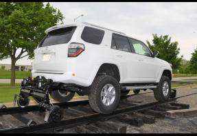
Mitchell model 1515 Flexiride Rail Gear for Toyota 4-Runner. Vehicle shown with 3 inch lift kit, heavy duty shock absorbers, reversing railroad lighting, upgraded 285/70R17 All Terrain Type, load Range E tires, composite rail wheels, in-cab controls, electric locks, and rail shunts.
